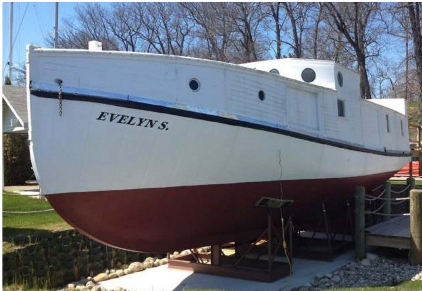
Color example of metal clad haul with wood cabin above.
