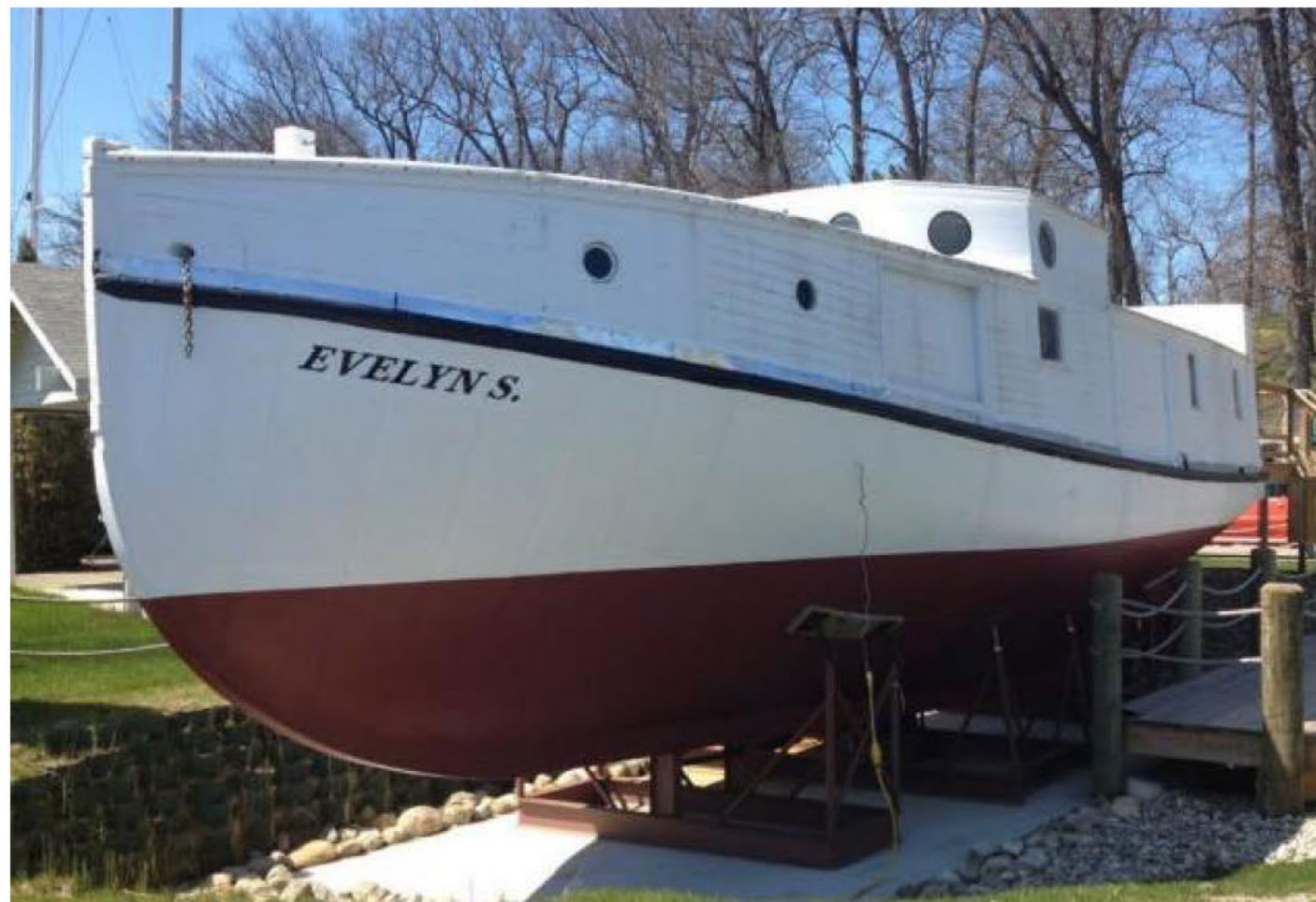
Color example of metal clad haul with wood cabin above.
